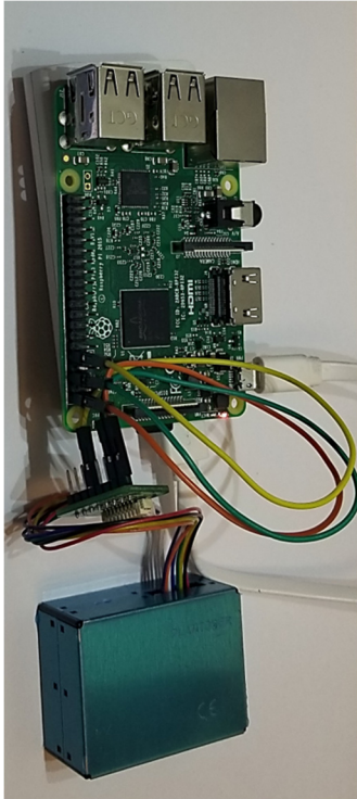
Figure 2: The mobile sensing module of myCityMeter is a wireless embedded sensing system with a computation and communication architecture based on the Raspberry Pi 3b+. It is a single board computer with a Bluetooth module, Wi-Fi, 1GB RAM, and 16GB storage. An off-the-shelf particle concentration sensor, Plantower PMS 5003, is mounted on the Pi along with a USB Power Bank (5V, 1A).
